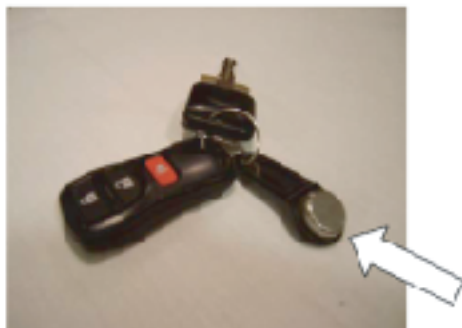
Fig 1: Key fob for the EMS vehicle driver to engage onboard monitoring and feedback device
